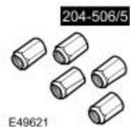
Retainers - halfshaft remover/replacer 204-506/5 (LRT-60-030/5)
